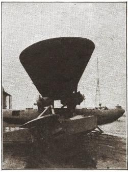
A contrast in the types of planes tested by the Navy. The large craft is a patrol plane (P3M-1), while the small ship alongside is designed to be operated from a submarine. The wing of this ship can be quickly attached and detached, and the whole machine can be stored within a special compartment inside a sub.
